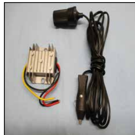
Cigarette lighter extension cord that was used shown alongside the step-Up converter.
