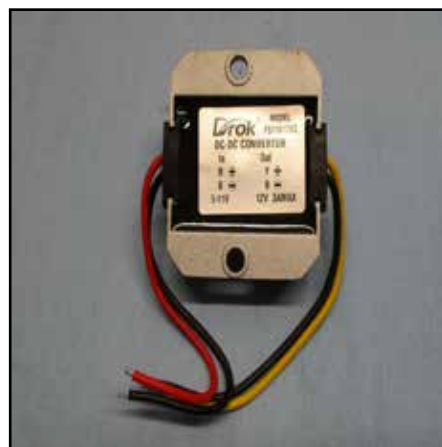
Step-up converter that I purchased showing simple wiring detail.
