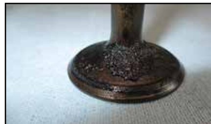
A small amount of oil coking on the backside of an intake valve.
