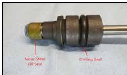
One-piece guide shown with the valve stem seal installed to the left and the O-ring seal installed around the guide O.D.
