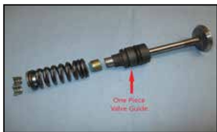
One-piece valve guide design introduced in about 1949.
