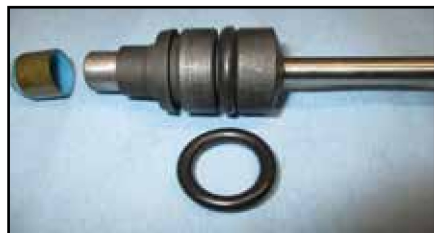
The large O-ring shown was also added to the one-piece guide to prevent oil from being pulled around the O.D. of the guide. A valve stem seal is shown to the left.
